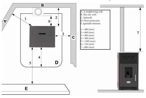
Mareli Systems **CHECK ITEMS BEFORE INSTALLATION** Chimney exit Chimney Connection to chimney **Connection to** the stove Security The chimney revision door distances
