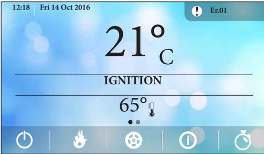
Blocking or non-blocking error is highlighted with a ! and the related error code. When pressed the error window opens
