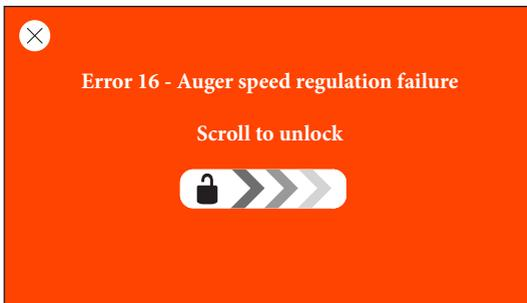
When this message is on screen this means that the product is in blocking mode and you can remove the error. You can do this by swiping to the right in the center of the screen.
