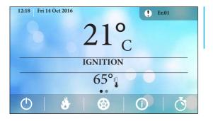
Blocking or non-blocking error is highlighted with a **1** and the related error code. When pressed the error window opens
