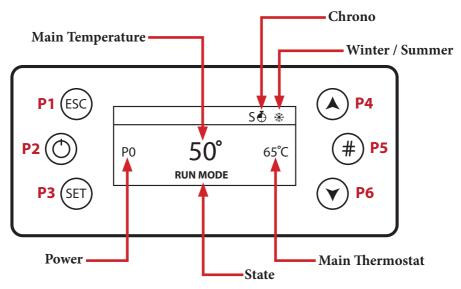
**P1** - Exit from menu/submenu refill Function (push for 3 seconds)
